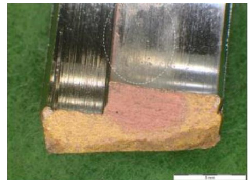
Failed nut showing some signs of coating removal and corrosion at point of a stress fracture (pink area)
