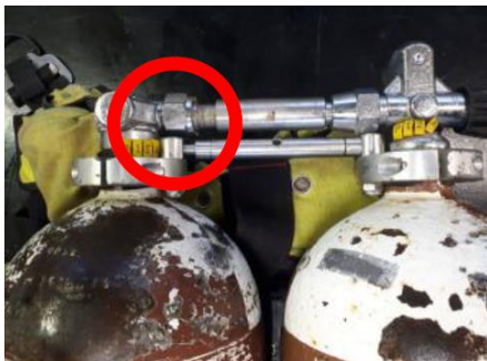
Bailout manifold assembly example showing location of failed nut
